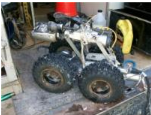
Pipe Inspection Robot
